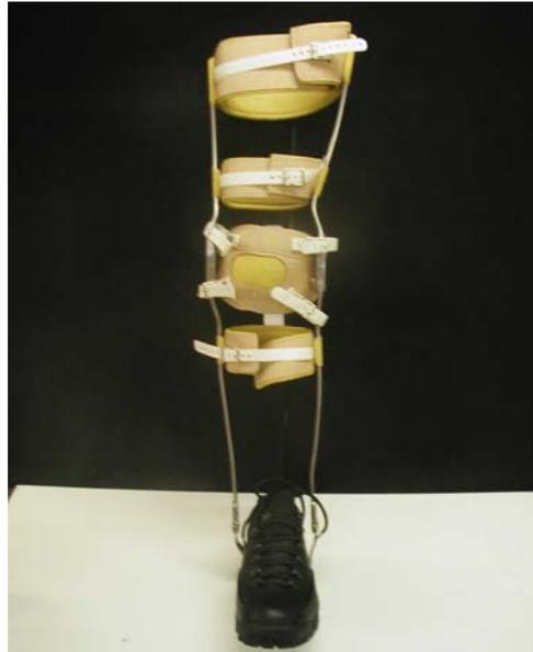
This "Conventional", "Double Upright" design of Knee Ankle Foot Orthoses (K.A.F.O.) is fabricated using a metal stirrup, metal ankle joint(s), metal knee joint(s), metal upright(s), metal band(s) and range of motion (ROM) locking hardware as required. These components are commercially available and are manufactured for specific conditional orthotic management.
