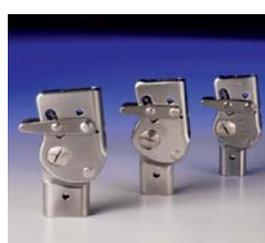
**Step Lock Knee Joints:** Similar to the Spring Lock Knee Joints accepting an integral step locking action upon extension resisting flexion in most requirements. ROM dependent on manufacturer. Lock out for full ROM present in quality manufactured components. Consider Cable System?
